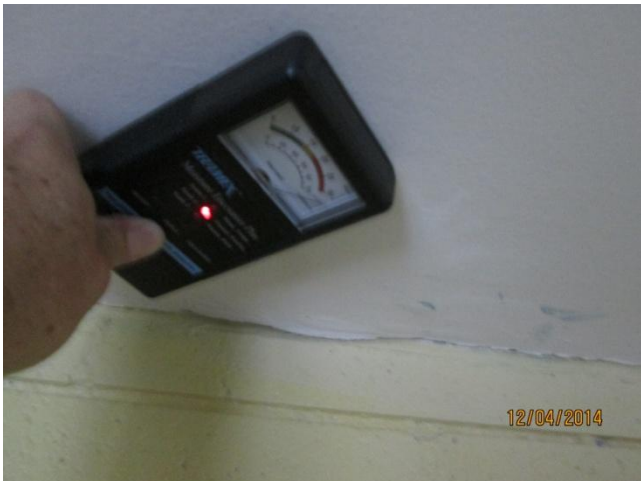
Laundry room ceiling showing water damage and blistering and wet readings on meter.
