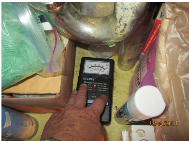
Under sink in bathroom elevated moisture levels and poor drain pipe condition appears to be leaking.
