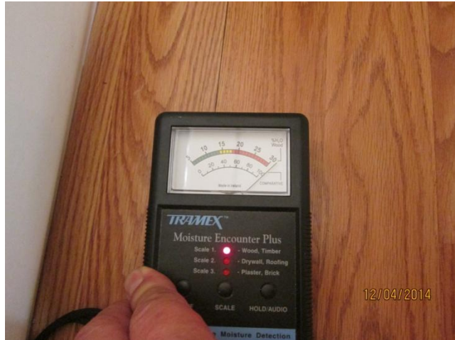
Inside cabinet shelf has standing water. Laminate floor next to tub and around toilet to cabinet is wet.
