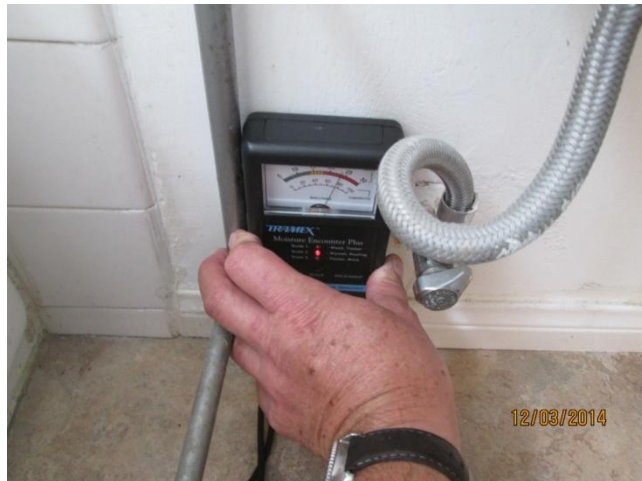
Cracks in tile surround for tub, elevated moisture levels in wall between tub and angle stop.
