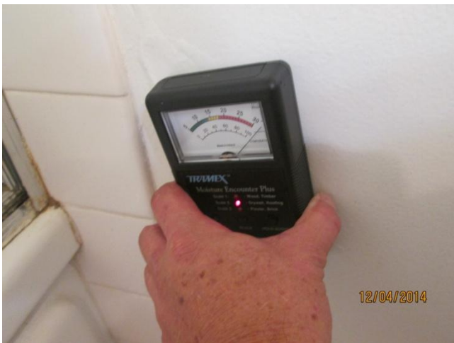
Elevated moisture levels going up 2' from floor to side of tub enclosure in bathroom. Dining room ceiling has repaired crack running the width of the ceiling.
