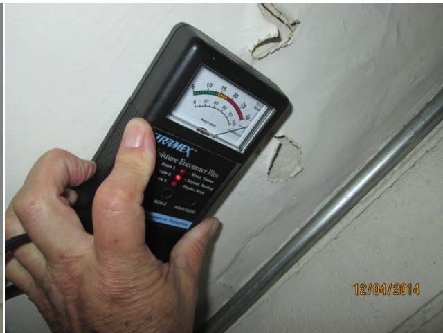
Laundry room ceiling showing water damage and blistering and wet readings on meter.
