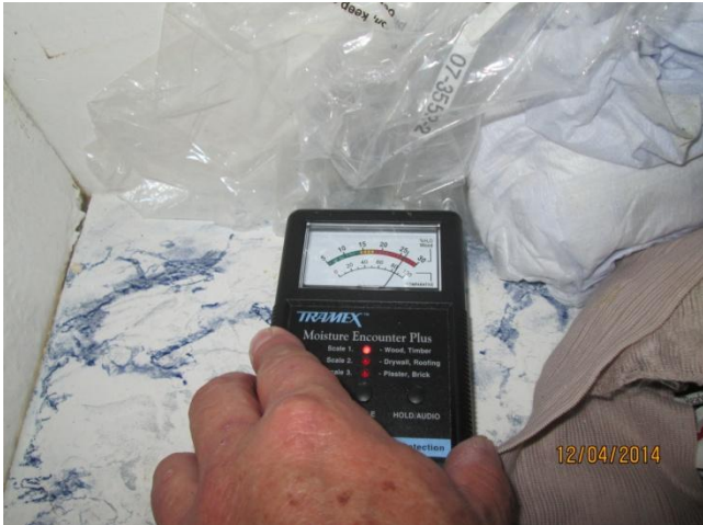
Sink cabinet in bathroom has wet shelf and side panels. Particle board is damaged.
