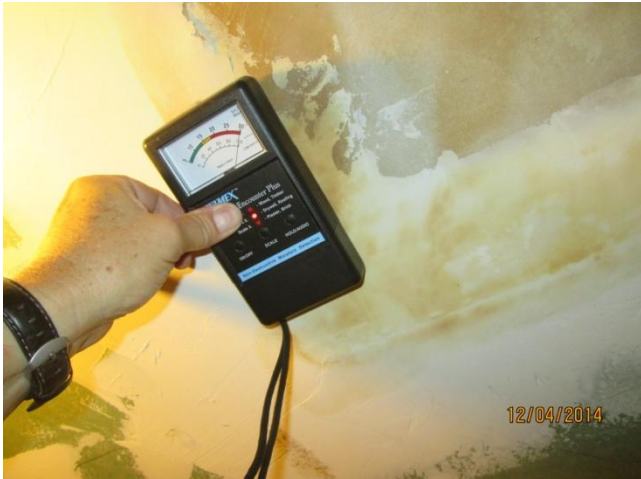
Water heater room ceiling is wet as shown by the meter readings. Entire ceiling is water stained.
