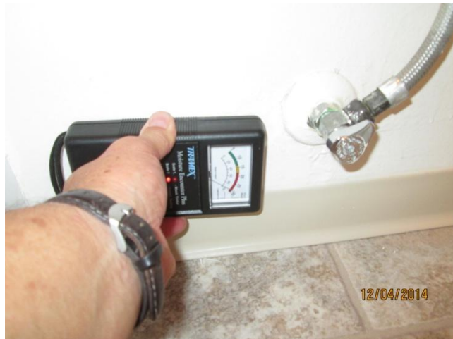
Inside cabinet shelf has standing water. Laminate floor next to tub and around toilet to cabinet is wet.
