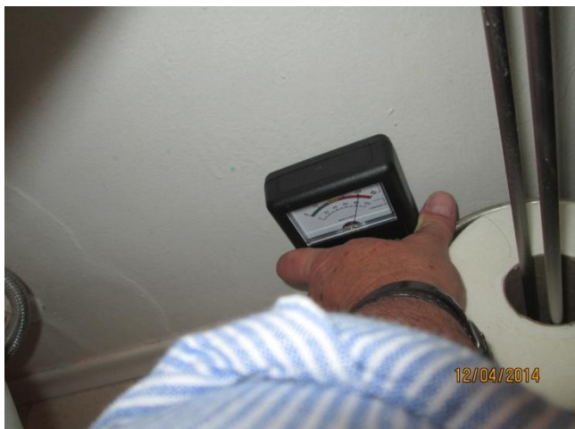
Elevated moisture levels found to right of tub on wall behind toilet. Living room ceiling has a repaired crack running the width of the room.
